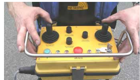
Portable control panel
