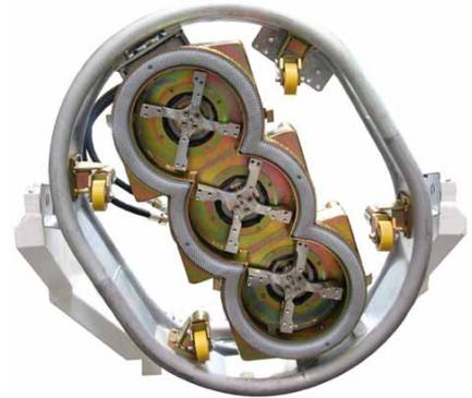
The blasting head can be swivelled so that both horizontal and overhead surfaces can be cleaned.
