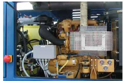
The hydraulic installation comprises two independent circuits each powered by a pump. The system is controlled by proportional valves, solenoid valves, pressure limiting valves combined with hydraulic motors and hydraulic cylinders. The hydraulic pumps are driven by a water cooled CAT diesel engine.
