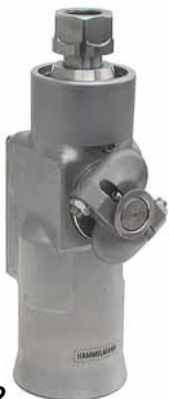
Type L 1400-2 with sledge for cleaning pipes with bends 35 mm S-arm, 2 nozzles max. 1400 bar / 150 l/min. Min. Pipe -Ø: 210 mm
