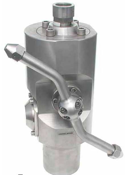
Type XXL 1600-2 56 mm lever arm, 2 nozzles max. 1600 bar / 500 l/min. Min. Tank access: 300 mm
