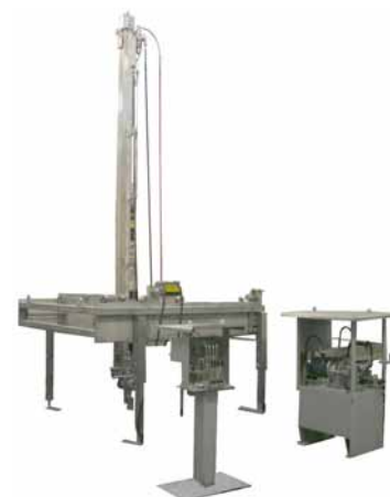
Pipemaster with operator's control station and hydraulic power pack
