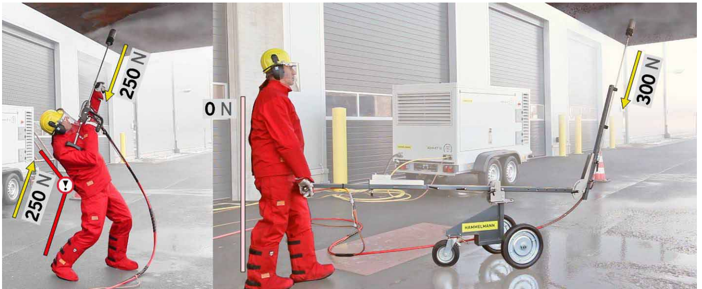
Manual blasting gun work
