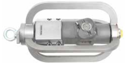
Type XL 1600-2 with sledge for pipe cleaning 35 mm S-arm, 2 nozzles max. 1600 bar / 250 l/min. Min. Pipe -Ø: 320 mm
