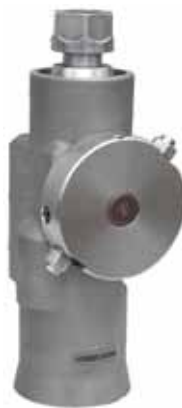
Type XL 1600-2 13 mm V-arm, 2 nozzles max. 1600 bar / 250 l/min. Min. Tank access: 190 mm
