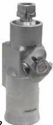
Type L 1200-2 with sledge for cleaning pipes with bends 35 mm S-arm, 2 nozzles max. 1200 bar / 150 l/min. Min. Pipe -Ø: 210 mm
