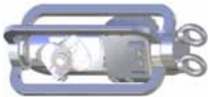
Type L 1200-2 with sledge for cleaning pipes with bends 35 mm S-arm, 2 nozzles max. 1200 bar / 150 l/min. Min. Pipe -Ø: 210 mm
