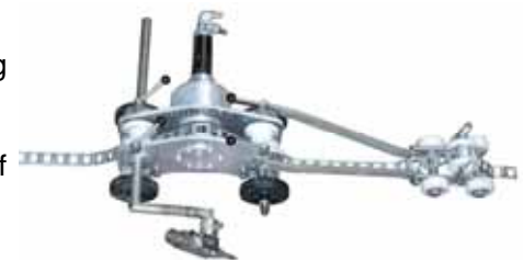
Carrier trolley with tensioning trolley
