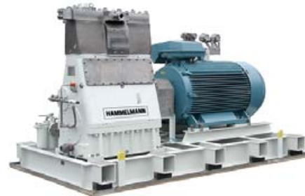
HDP 555 pump unit for glycol and methanol duty Op. pressure 10,700 psi – 740 bar, Flow rate 87 gpm – 333 l/min
