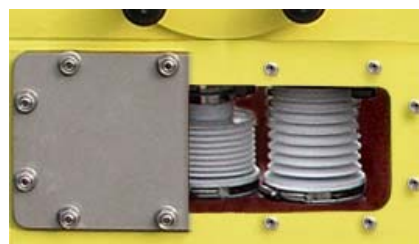
The bellows system is gastight.
