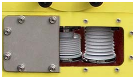
The bellows system is gastight.
