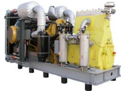
Typical high pressure pump units
