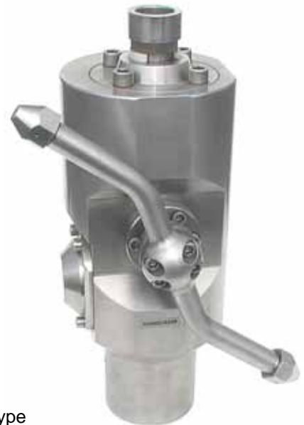
Type XL 1600-2 with sledge for pipe cleaning 1.38 inch S-arm, 2 nozzles max. 23,200 psi / 66 gpm Min. Pipe -Ø: 12.6 inch
