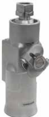
Type L 1200-2 with sledge for cleaning pipes with bends 0.71 inch S-arm, 2 nozzles max. 17,500 psi / 53 gpm Min. Pipe -Ø: 8.27 inch
