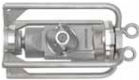
Type L 1200-2 with sledge for cleaning pipes with bends 0.71 inch S-arm, 2 nozzles max. 17,500 psi / 53 gpm Min. Pipe -Ø: 8.27 inch
