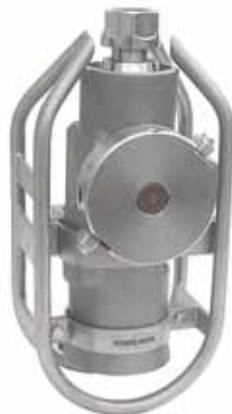
Type XL 1600-2 0.51 inch V-arm, 2 nozzles max. 23,200 psi / 66 gpm Min. Tank access: 7.48 inch
