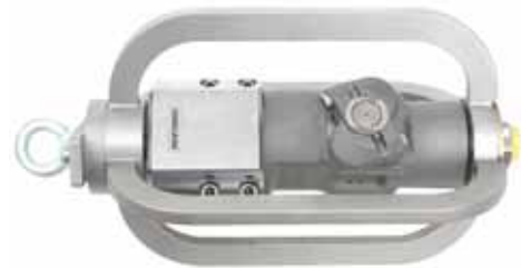
Type XL 1600-2 with sledge for pipe cleaning 1.38 inch S-arm, 2 nozzles max. 23,200 psi / 66 gpm Min. Pipe -Ø: 12.6 inch
